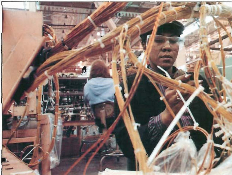
Douglas Aircraft technician sets up completed wire assembly for analysis and testing.
