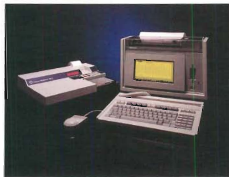
Combining software from HP Genenchem with the Integral PC, TiterCalc automates the data processing of microtitration in biotechnology laboratories.
